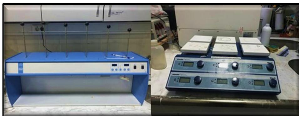
Figure 1 Laboratory scale Jar Test setup
